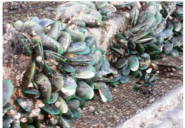
Figure 6. Filter from a power plant fouled with green mussels.
